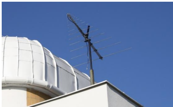
Figure 1. A log-periodic antenna CLP-5130-2N for the CALLISTO in Hurbanovo.
