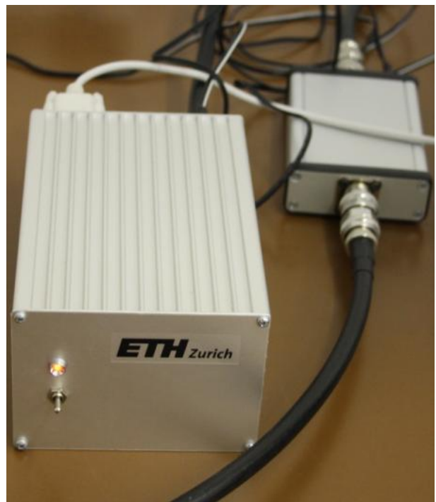
Figure 2. CALLISTO instrument No. eC50 (left) with the amplifier ZX60-33LN+.
